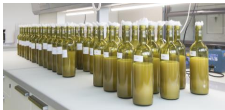
Figure 1: Fermentation experiences of Chasselas must (YAN = 95 mgN/L) using different yeast strains ( Sacch. cerev. ) without (Control) and with 200 mgN/L (NH_4)_2HPO_4 supplementation.
